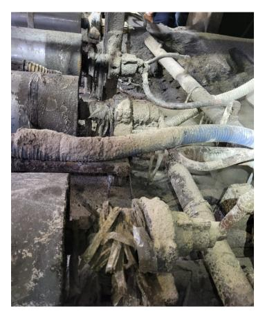
During the second visit, Enviropeel engineers completed a range of new applications and inspected all the previously completed work. Despite the conditions, all the bearings were in perfect condition.
