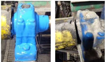
Photos on the left show the condition of an array of bearings prior to application and the same bearings after application. Above, a freshly-completed bearing from a similar area is shown next to the same bearing after just a few weeks of exposure.
