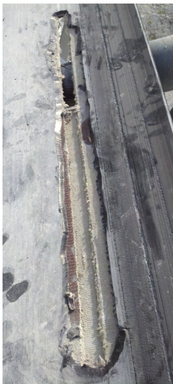
The photo above shows the severe damage to the belt. On the right, the same area of the belt is shown, following repair with Rubberloc
