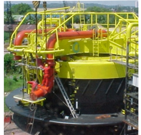
Before and after: left, the main buoy during preparation before coating. Above, after the coating works are complete.
